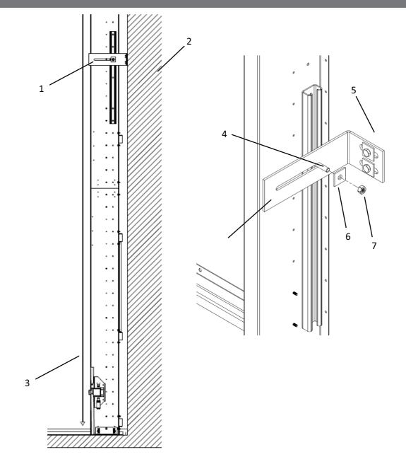
Figure 12, Fixing the guide frame against the building wall
